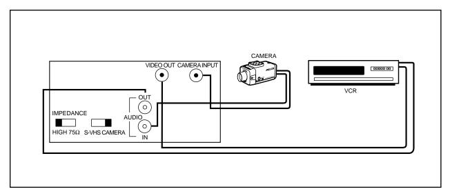
Figure 2. One Monitor with External Video Equipment
